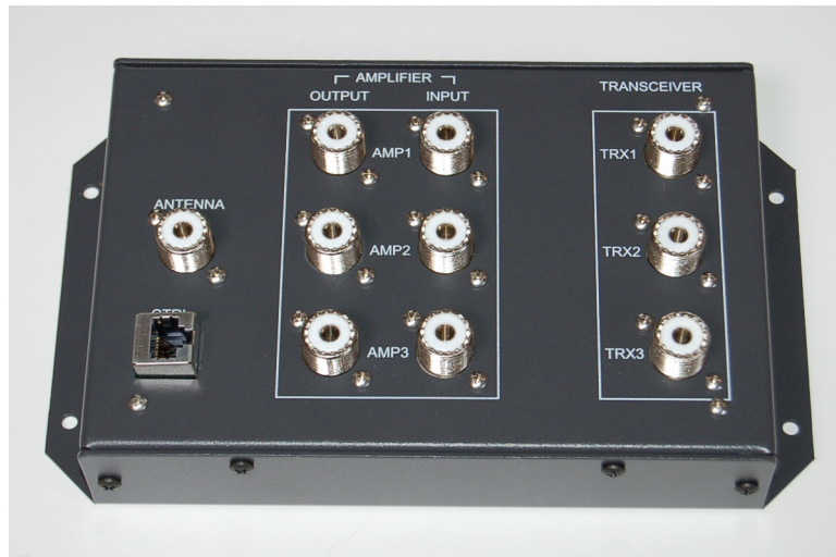
The completed StationPro RF relay unit
